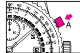
2. Stop the measurement by pressing pushpiece A once more. The measurement is done in hours (totalizer 1), minutes (totalizer 2), seconds and  $\frac{1}{5}$ ths of a second (hand 3).
