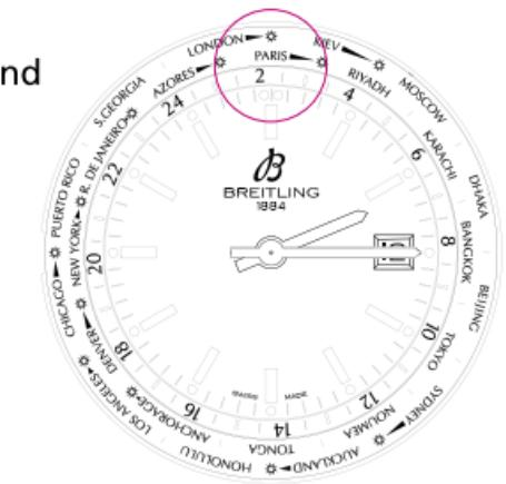
3. Pull the crown out to position 3 – the watch stops to enable setting to the nearest second. Turn the hands forwards or backwards to adjust the hour and minute while taking account of the 24-hour disk indication and being careful not to move past midnight in order to avoid the date jumping.
