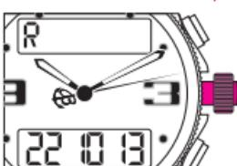
The respective synchronization of analog H, MIN and SEC (hands) is done by rotating the crown. N.B. The SEC only move clockwise.
