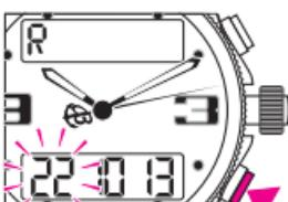
Press pushpiece B briefly: the hours, minutes and seconds (H, MIN and SEC) of the display each flash in turn.
