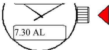
[image 37-5] when the alarm sounds, press on the crown to end the buzzing.
