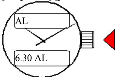
[image 38-3] To test the alarm function, press on the crown during more than two seconds after selecting the alarm (AL) function: the buzzer will sound.
