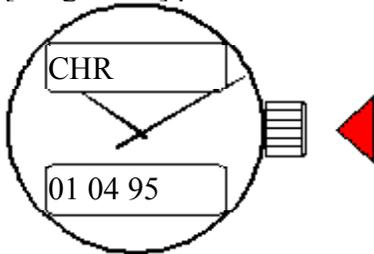
[image 35-4] a further press on the crown will restart the chronograph, allowing a series of short times to be measured and added together;
