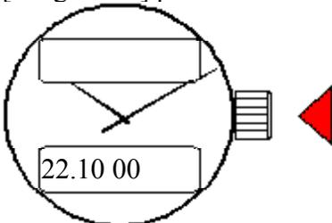
[image 27-2] while the seconds digits flash, push the crown back in precisely at an observatory time signal or when a reference time source marks the exact minute: this will return the seconds digits to zero [and the minute digits to the nearest minute].
