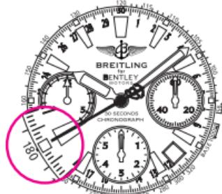
*Example 2:* if it takes 36 seconds to cover one kilometer or one mile, the average speed is 100 km/h or 100 mph respectively.
